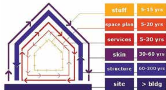
Figure 2 Building layers according to anticipated lifespan (Brand, 2004)
